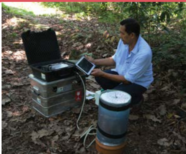
Researcher Roberval Lima operates a device designed to measuring soil respiration
